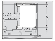
8 Be sure that the stack of paper fits completely under the latches of the side guides.
